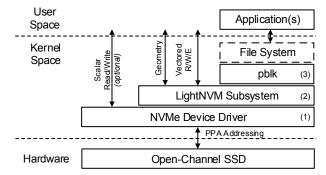
Figure 2: LightNVM Subsystem Architecture
